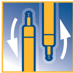
Installation position any as required Einbaulage beliebig
